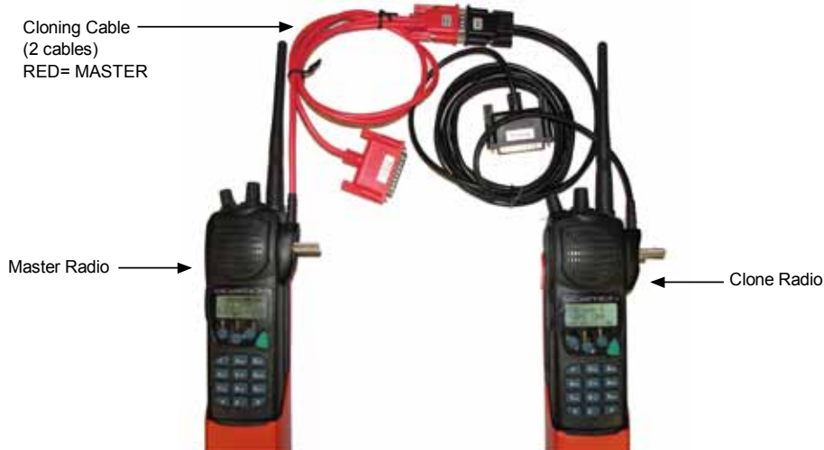
Fig. 8: Cloning Cable Connections
