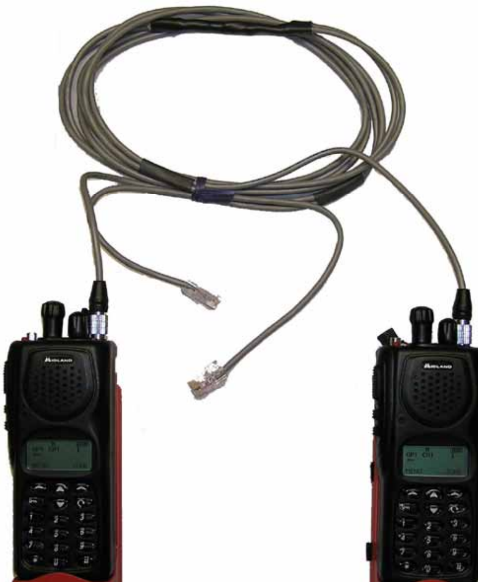
Figure 8: Midland Cloning Cable Connections
