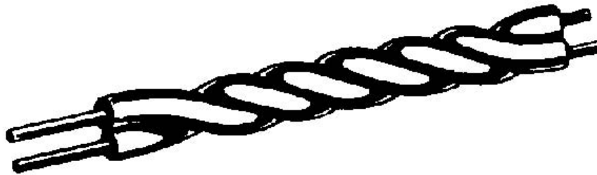
Figure 1-20.—Twisted pair.
